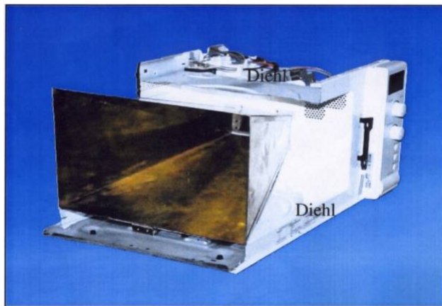
MODIFIED microwave oven weapon for improved focus of the microwave radiation
